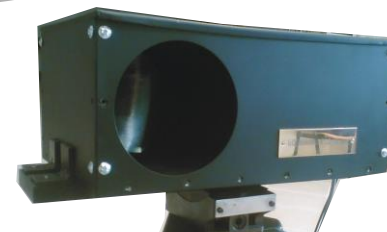
Constructed FSO receiver
